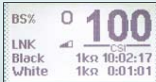
Sensor impedance indicators, CSI, BS%, case monitoring time and link signal indicator.
